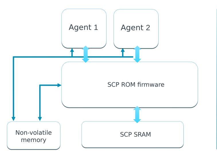
SCP ROM firmware gets the SCP RAM firmware image from an agent or from non-volatile memory, loads it into SCP dedicated SRAM and passes control to the SCP RAM firmware image.
